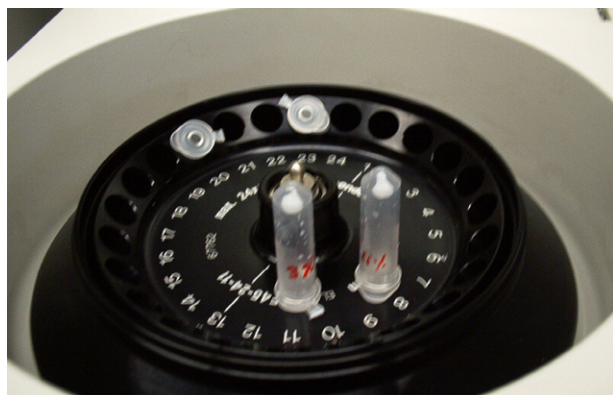
Figure 1. Two-milliliter volumes of the emulsions were centrifuged for 30 minutes at 16,000 g to remove large aggregates formed during the polymerization process. The compacted pellet obtained after removal of the supernatant is shown.
