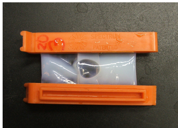
Figure 2. Dialysis of the emulsion was conducted with different dialysis membranes (MWCOs of 6–8K, 12–14K, 50K, and 100K) and dialysis times (4–24 hours) in bulk water.
