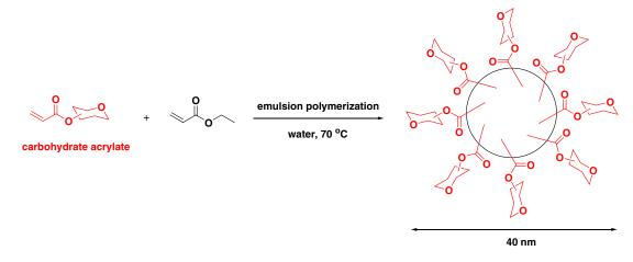
Scheme 1. Synthesis of glyconanoparticles by emulsion polymerization.
