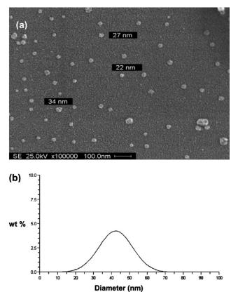
Fig. 2. (a) SEM image and (b) particle size distribution of glyconanoparticles prepared from 3-O-acryloyl-1,2:5,6-di-O-isopropylidene- $\alpha$ -D-glucofuranose (1) and ethyl acrylate by emulsion polymerization.
